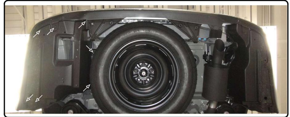
2. Remove the (4) rubber plugs from the frame rails and unscrew the (5) threaded plastic inserts from the frame rails. Return plugs and inserts to owner.
