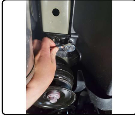
5. Lower muffler by removing exhaust hanger rod closest to the exhaust tip from rubber isolator. Reinstall in STEP 7.
