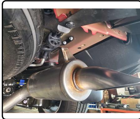
6. Raise the hitch over the exhaust and align the holes in the hitch with the weldnuts in the frame. Secure the hitch to the frame using the supplied M12-1.25 hex bolts and 1/2" conical toothed washers. Torque all 12mm hardware to 86 ft-lbs.
